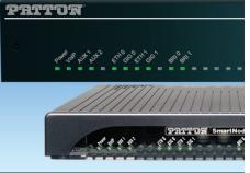
The SmartNode 5530, is a cost effective eSBC with integrated Broadband access and up to 8 BRI ports supporting a high level of VoIP and network security. It is capable of doing up to 200 SIP to SIP calls\*\*\* whereof max. 8 can be transcoded\*\*. Built-in QoS functionalities and support of G.722 high definition codec, ensure excellent VoIP call quality.
